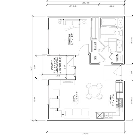
UNIT C1 (1) BED UNIT FLOOR PLAN GROSS AREA: 1103 SQFT NET AREA: 817 SQFT BALCONY: 61 SQFT
