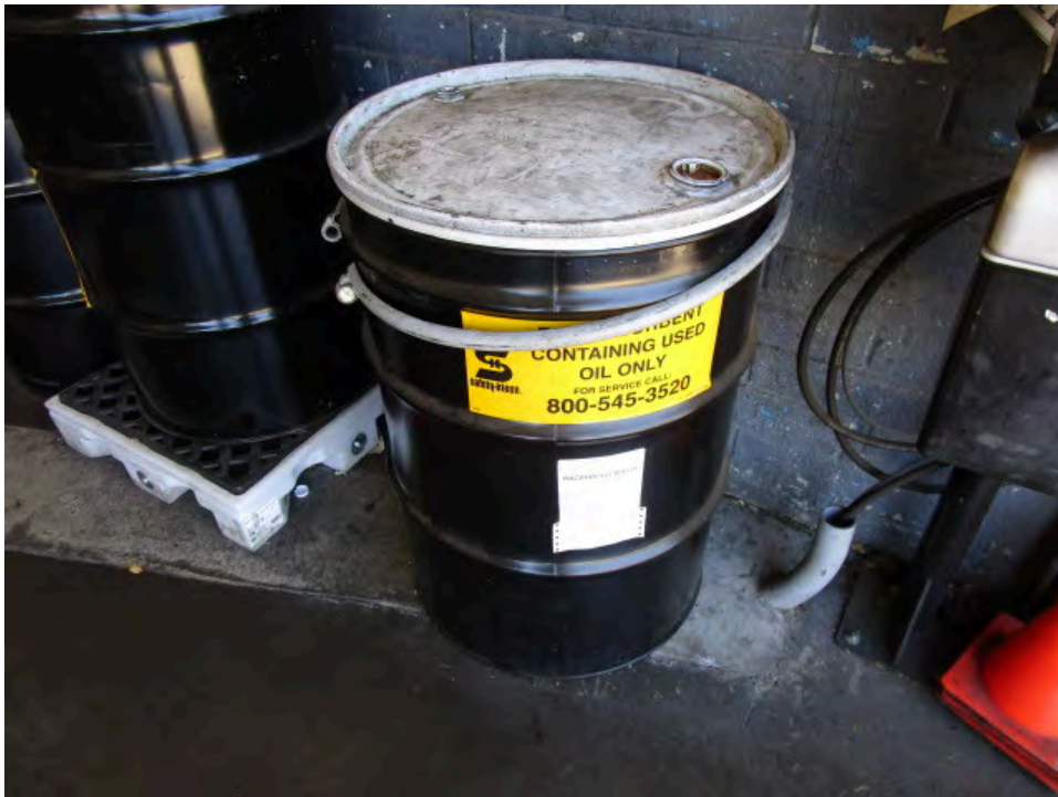
20. 55-gallon drum with oil-containing absorbent
