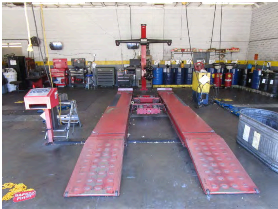
24. Alignment rack in the automotive service area
