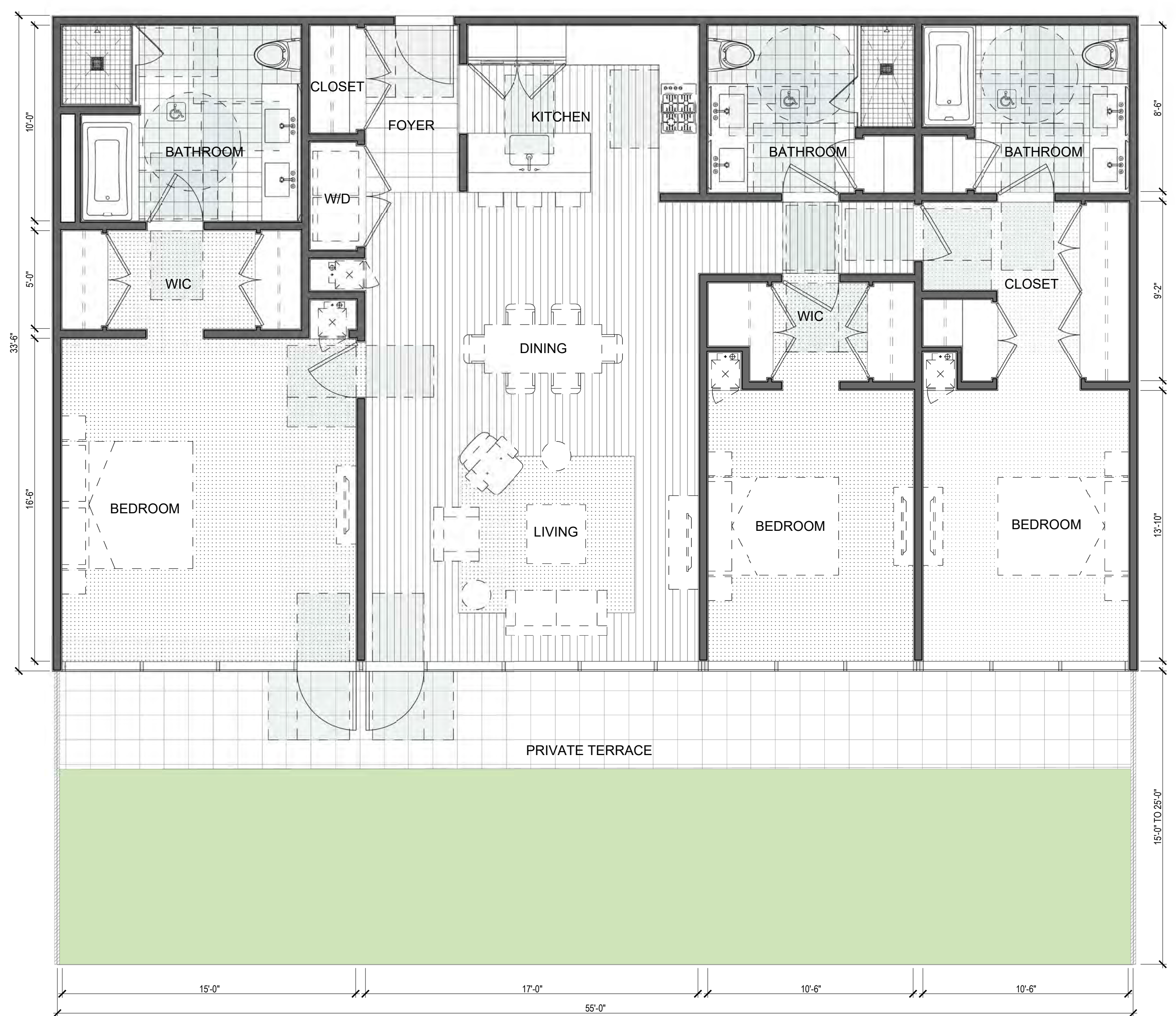
ENLARGED UNIT FLOOR PLAN - 4 BEDROOM TERRACE UNIT (2177SF) TRC 1/4"=1'-0" 3
