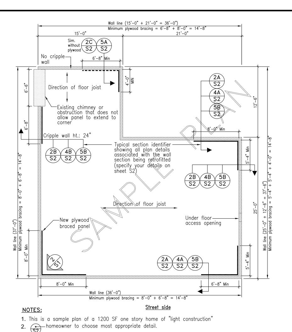
SAMPLE FOUNDATION AND PLYWOOD LAYOUT PLAN TECHNICAL NOTES SCALE: 3/16"=1'-0"
